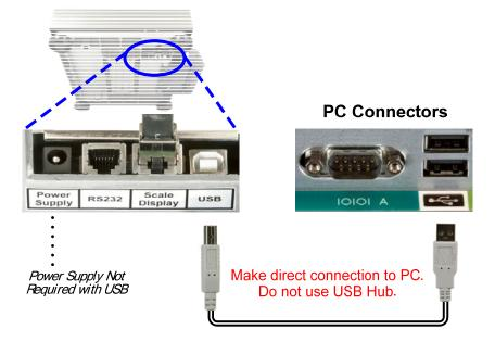
Check for USB communication by verifying the scale is properly connected to the PC through the Device Manager utility in MS Windows. Access the Device Manager (XP operating system is shown below) by clicking Start – Settings – Control Panel – Systems. In Systems, click on the Hardware tab, than the Device Manager box.
